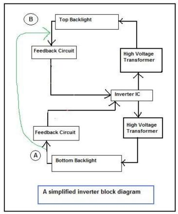
I know that it is a bit confusing about this configuration but once you have understood how this circuit work, you then can know whether the LCD Monitor display shutdown problem is caused by a faulty backlight or the inverter circuit itself.
