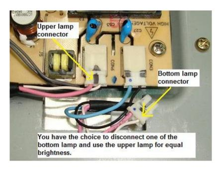
Note: I do not encourage you to modify the circuit with one high voltage transformer to power up four lamps (top and bottom) as this will overload the transformer and the related circuit.
