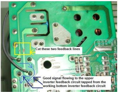
Once you have tapped the two feedback signals, it is time for you to switch "ON" the Monitor. Yes, it worked perfectly good without the display shutting down due to now there are feedback signals (which were tapped from the bottom lamp feedback circuit) flowing to the inverter IC. Even if the upper (top) lamps disabled (not connected) the inverter circuit is still functioning!
