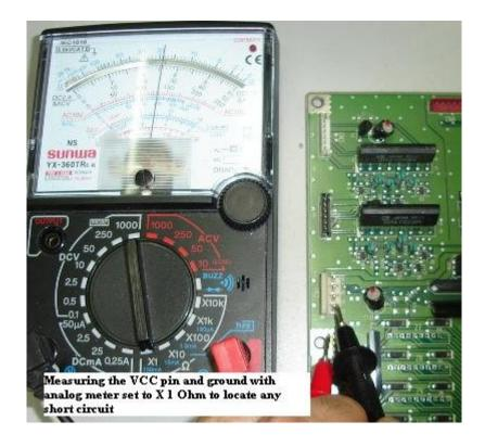
If you have confirmed that the 5 volts line have problem then how do we find out the culprit since there are so many components connected to this line? TTL IC's, CPU, EEPROM, transistors, diodes and even small filter capacitors are all connected to the 5 volts line. Either one of these components shorted could cause no power to the printer.
