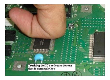
Why don't I immediately turn the output voltage from the dc regulated power supply to 5 volts since the defective main board is also using 5 volts to run? If I do this and if the faulty components turned hot too fast, I'm afraid this will lead the faulty component to open circuit. If the faulty component open circuit, the current draw will drop and the only clue that you have to identify the culprit has been destroyed!
